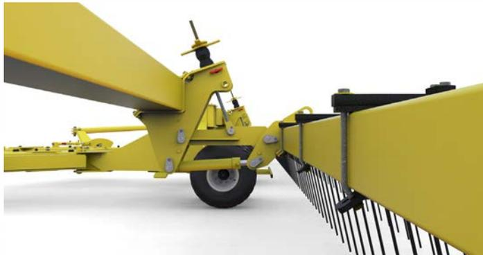
transfer the machine weight to each tine, but it does so in hilly conditions. In float position or under pressure, the harrow sections are designed for flexibility. The torsion spring bars are positioned along the sides of the harrow frame providing an even distribution of pressure to the frame.
