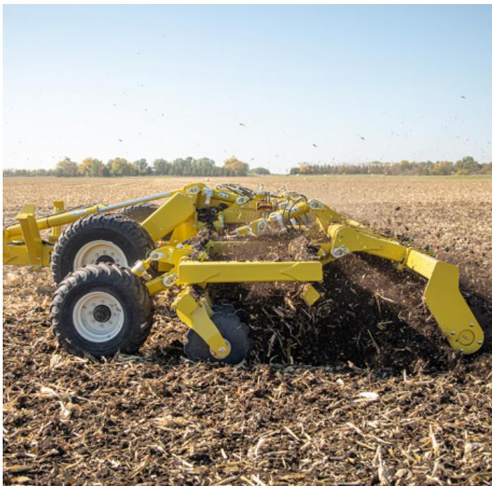
With the Pro-Till 20/26, Degelman Industries is able to offer the same high-speed, high-performance discs as our three-plex machines in a size that fits the 300 – 450 HP range, all without sacrificing our frame size, or the average weight per foot. In addition, we made the 20/26 Ft Pro-Till our first ever, completely greaseless, maintenance-free machine. It's true "drop the pin and go" mentality.
