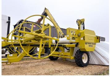
bag is lifted and pulled onto the drive spools, it is gently guided into place by the RENN roller and hold down system – reducing stress on the bag and helping prevent spillage. RENN's continuous-flow unloading system effortlessly draws the Unloader and power unit into the bag, while quickly unloading the bag contents through high-capacity discharge augers.
