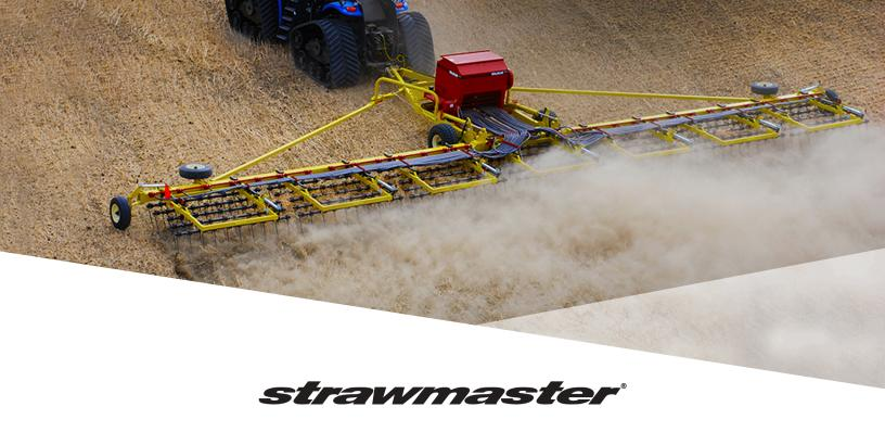
With 26 inch long times equipped with tungsten carbide tips placed in five rows, and set in large ten foot wide by six foot deep sections, this machine is at the forefront of modern straw management.
