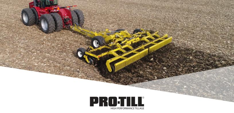
The fastest and most versatile piece of tillage equipment you will ever own, the Degelman Pro-Till® shreds heavy fall residue, opens up spring fields, levels ruts, destroys clods and produces an absolutely perfect seed bed. Pro-Till® is your single tool for tillage.
