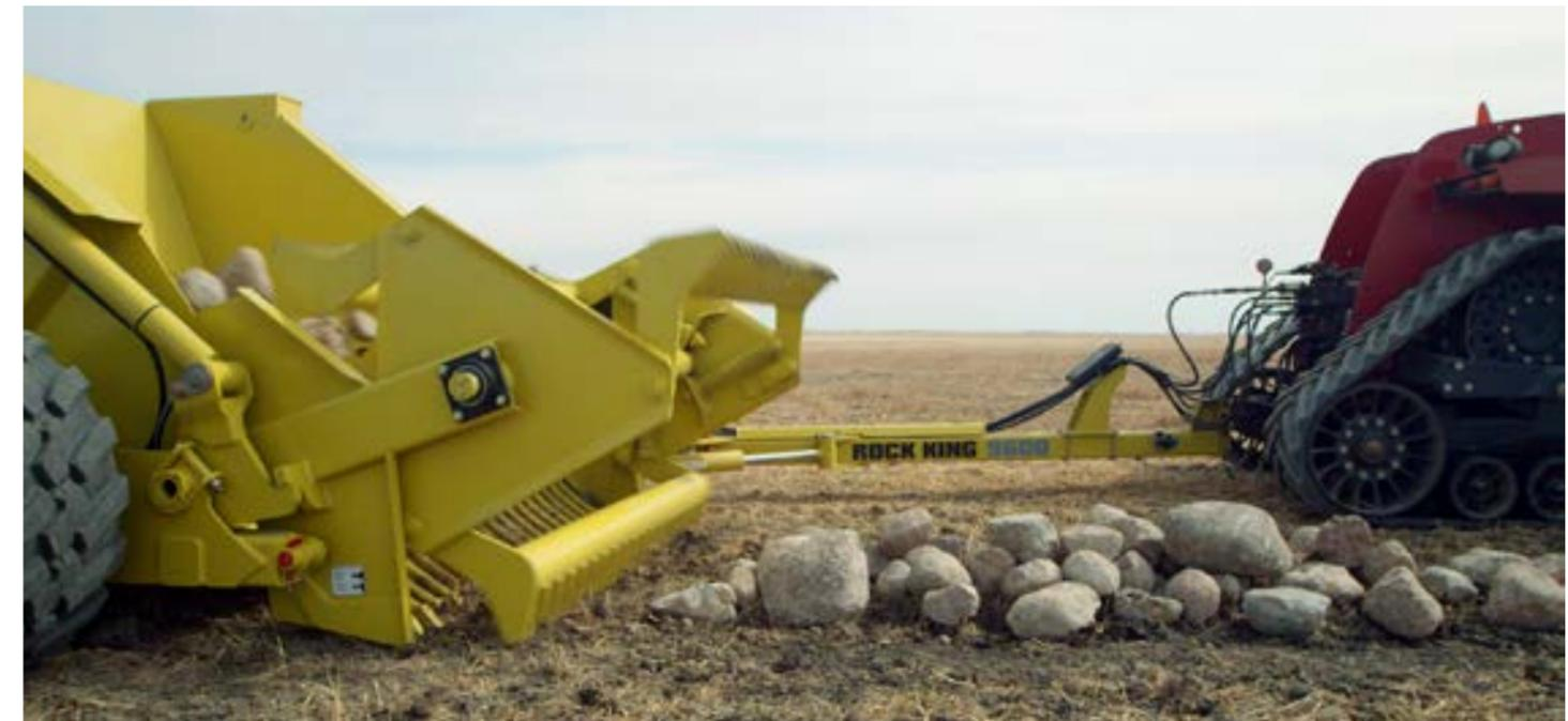
The unique interlaced grill and paddle teeth drop dirt easily onto the field. Even the bottom and rear of the hopper box make use of grated spring bar strapping to keep rocks in and dirt out.
