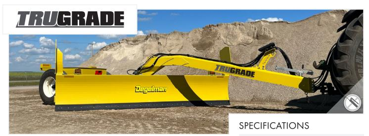
Introducing the Degelman TruGrade, the tallest pull type bulldozer blade on the market. Our streamlined design will make cleaning ditches, grading roads, digging ditches, leveling fields, and moving snow easier and more efficient than ever.
