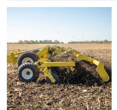
With the Pro-Till 20/26, Degelman Industries is able to offer the same high-speed, high-performance discs as our three-plex machines in a size that fits the 300 – 450 HP range, all without sacrificing our frame size, or the average weight per foot. In addition, we made the 20/26 Ft Pro-Till our first ever, completely greaseless, maintenance-free machine. It's true "drop the pin and go" mentality.
