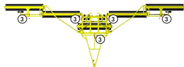
4) Slowly drive forward and wings should fall-back in line behind the center frame.
