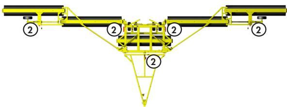
3) Activate these circuits again to allow cylinders to rest on the red transport bars.
