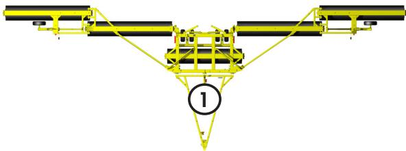
2) Fully extend the transport wheel cylinders to raise the rollers off ground and activate the hitch pole cylinder to allow installation of all five (5) red transport bars.
