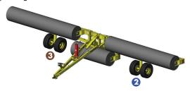
7) Backup until the wings are straight in line with the center frame. Ensure wheels are straight before Step 8.
