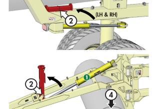
3) Activate the End Wheel Circuits 2 & 3 to turn each Endwheel to around 20° max. Try to match the angles on each wheel.
