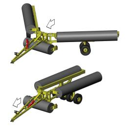
5) Install the cylinder transport bars onto both LH & RH endwheel cylinder shafts and secure.
