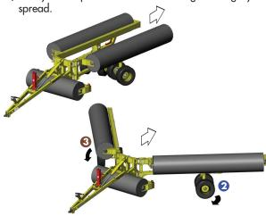
6) Turn the wheels 2& 3 while backing up. Avoid pushing on the sidewalls of the tires.
