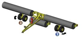
2) Slowly extend LH Endwheel cylinder 2 until the wheel is completely turned.
