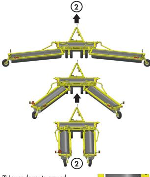
Lower drums to ground and slightly raise endwheel struts so wheels are off the ground.
