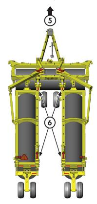
6) Install the four Red Transport Bars onto the End Wheel & Center Wheel cylinder shafts and secure in place using the lock-pins.
