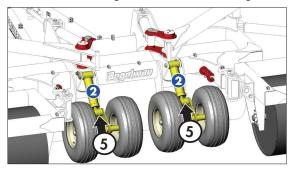
6) Remove the Red Transport Pin from the float hitch and secure it in storage position.
