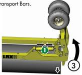
4) Continue activating this circuit 1 to fully extend the Power-fold Cylinders and open the wings. Ensure both of the Swing-Arm shafts latch properly into place.
