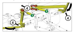
5) Retract the Center Frame Cylinders 2 to raise the center frame wheels (lowering the center section to the ground).
