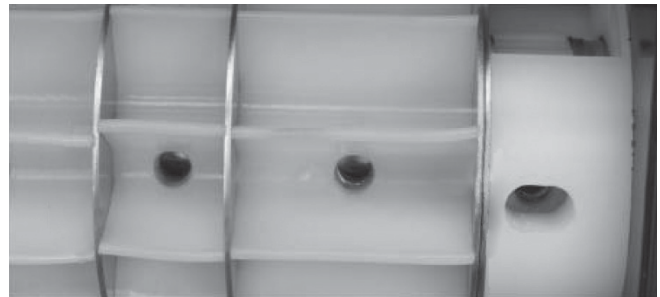
High compression: Wheel rib edges become curled/wavy.
