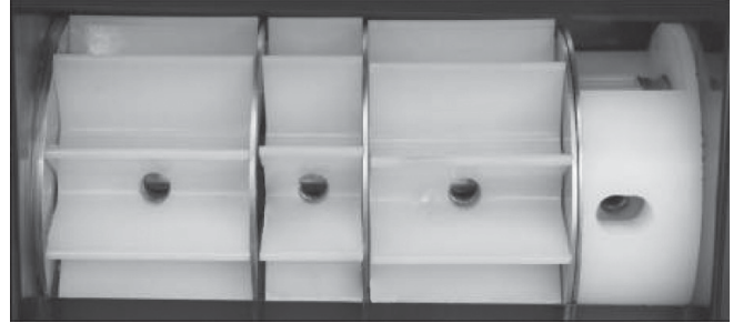
Low compression: Insufficient side pressure creates gaps.
