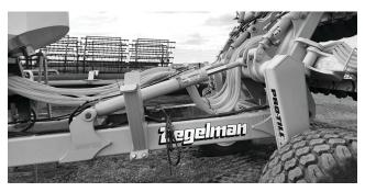
From here the hoses route down, under the center frame following a smooth, gradual curve into the **Wing Guide Brackets**.
