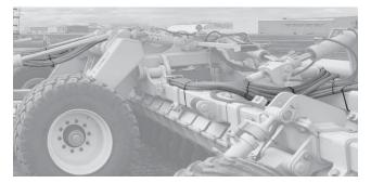
The hoses continue to the Wing Frame cross beam and then follow it to the rear of the machine.
