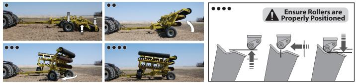
Transport Dimensions Height - 4m (13 ft) Width - 6m (20 ft) MAX Transport Speed 40-50 km/h (25-30 MPH)
