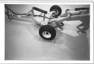
25. Hitch and pin the machine to tractor and install the hydraulic hoses to tractor outlets. Load up and cycle the hydraulic cylinders several times to remove any air in system.
