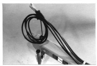
Install the four nipple fittings shown onto hose ends.
