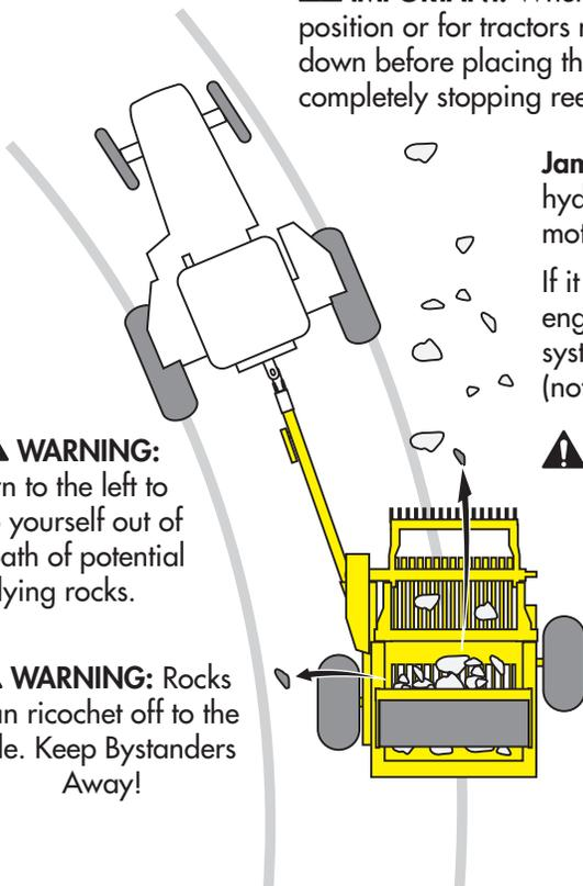
**Jamming/Unplugging:** After reel has completely stopped, move the hydraulic control lever the other direction to reverse the hydraulic motor. Reversing the reel will in most cases dislodge the jammed rock.
