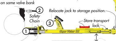
Adjust bolts and hitch position to set pole height.
